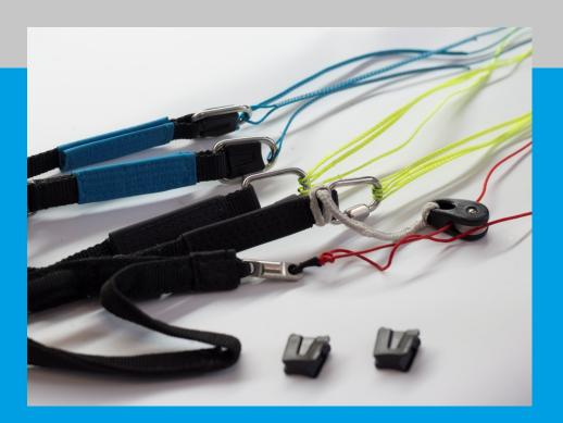
Check the line as it has two different loop sizes. First one we use the shortest loop to attach to the B riser.
