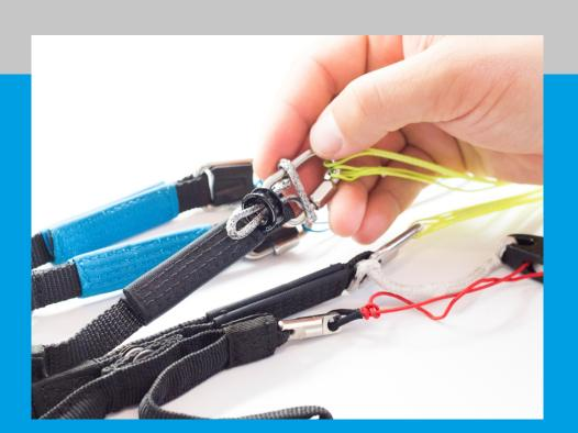
Flip the loop over the Tykaska O-ring and push the O-ring all the way trough the loop.
