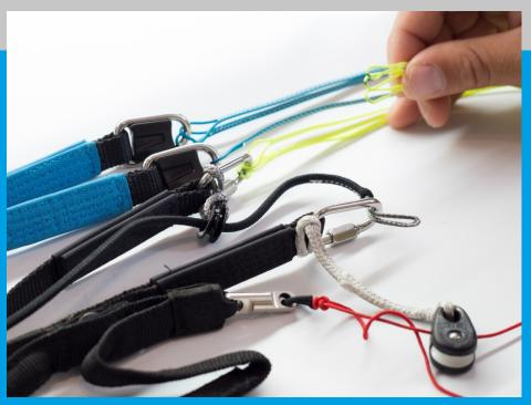
Flip the loop of the line over the carabiner. It is important that the line is travelling straight from B line trough the Tylaska O-ring and is finishing on the C riser from the front to back side.
