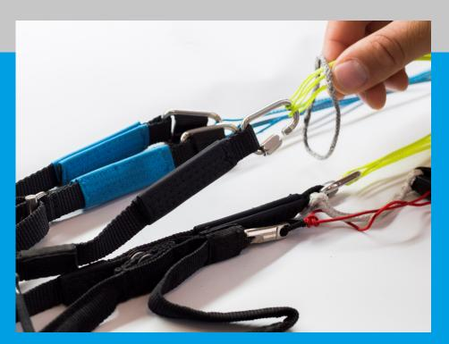
Drive the loop trough the carabiner as it is in the picture. It is very important that the remains of the loop are facing backwards towards the C riser.
