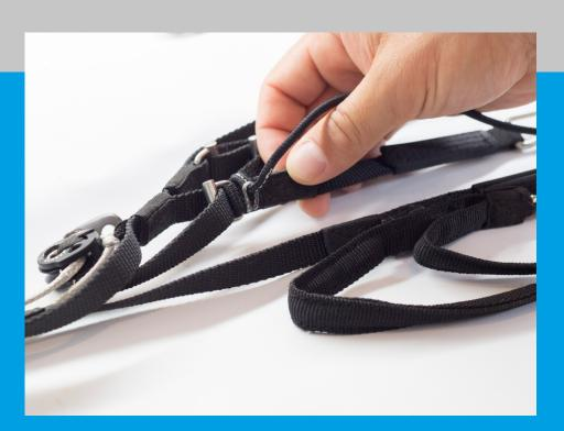
Before disconnecting all the lines, remember or write somewhere the settings you had with loops on the riser. After that, disconnect the lines on the B riser and use the loop in the package to drive the lines trough it.
