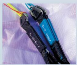
The line-set is greatly reduced; amazingly so for an EN A. There are just two main A-lines on each side, one going to the Big Ears riser and the other to the main one. The lines themselves are, as you would expect, sheathed and not super thin.
