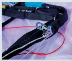
speedbar pulleys are the same sleek flat design as we saw on the Queen, and the two risers are colour coded at the bottom.
