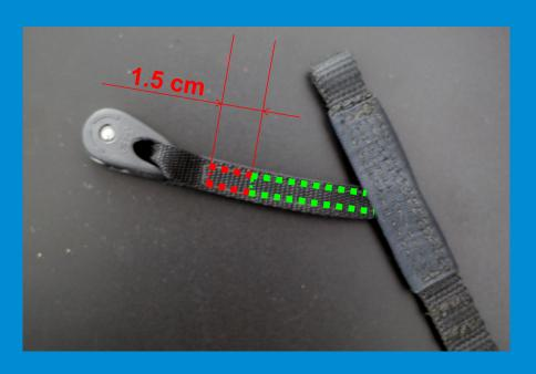
Delete the seam by 1.5 cm in order to make space for the loop of the new pulley.
