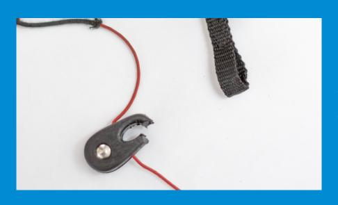
Take away the pulley, untie the brake line, detach it from the brake and pull the line out of the old roll. Take extra care, to have the lines sorted out all the time.
