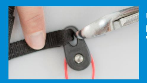
Use the clamps to cut trough the plastic pulley. Take great care to not damage the webbing of the riser.
