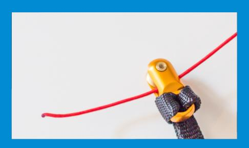
Once the pulley is attached pull the brake line trough exactly the same way as it was before. Connect the line to the brake handle properly.
